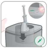
Warm syringe in syringe holder (available separately). Contacts of holder and device base connect. Lamp lights up green.
